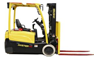
Active Mast Control monitors lift height and load weight, automatically reacting to limit or prevent tilt and reduce the likelihood of a tip over.
