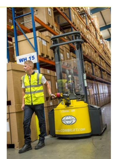
Incorporating the benefits of AC technology in its traction, pump and steering motors, the Combi-WR has a lift height that can be tailored to your application with load capacities up to 1,450kg.
